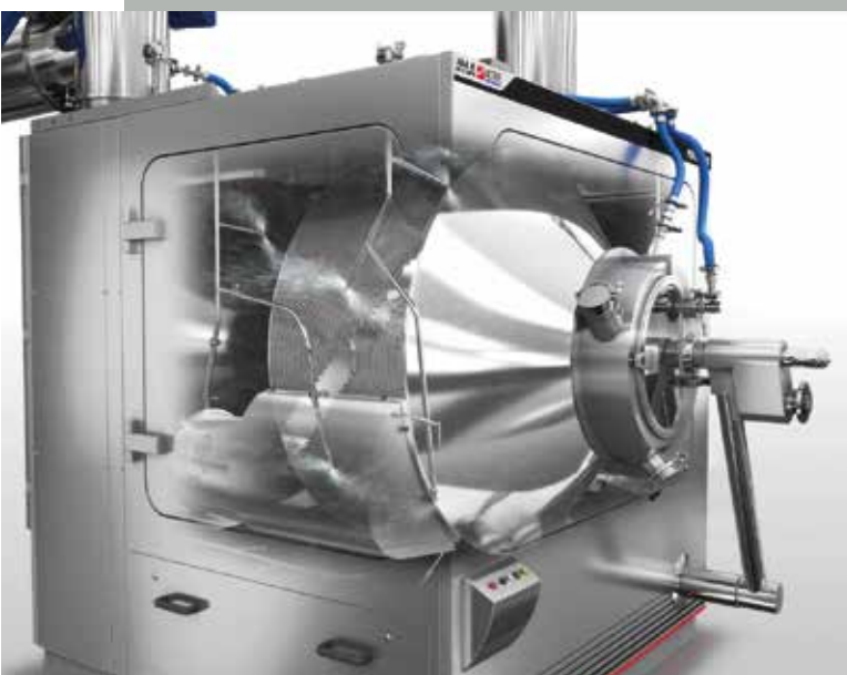
Figure 5: 3D model with details of "O" lines: rotating nozzle inside the PERFIMA cabinet
