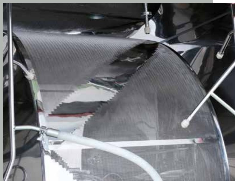
Figure 6: detail of "O" lines: rotating nozzle inside the PERFIMA cabinet
