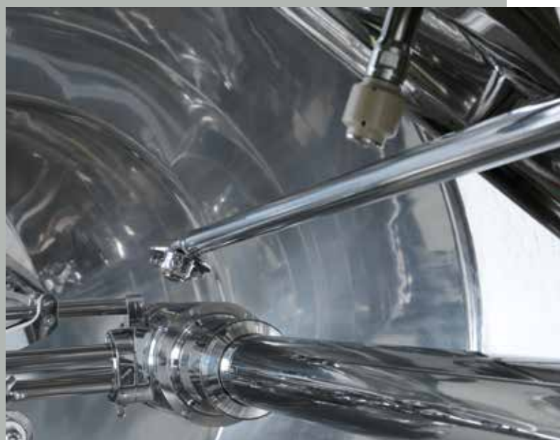
Figure 4: Detail of washing line I1: front rotating lance and front door rotating nozzle inside the drum
