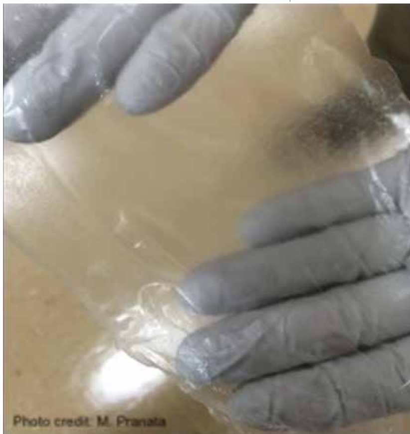
Figure 1. Egg white protein film obtained using extrusion and calendaring processes (Photo retrieved from Maruscha Pranata's thesis document).
