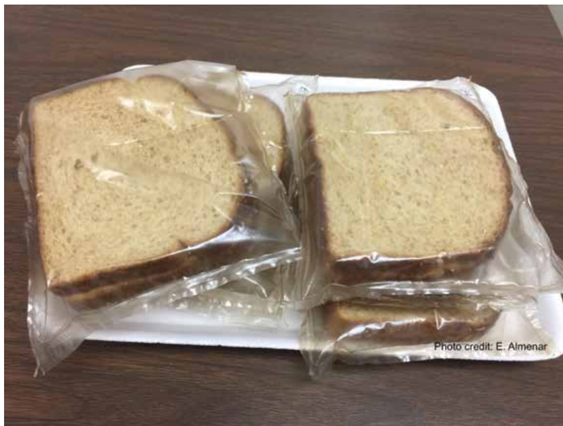
Figure 3. Sliced bread in pouches made of LLDPE/orange peel biocomposite blown at the MSU School of Packaging.
