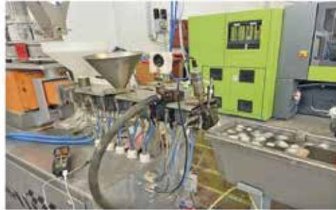
**Wet extrusion + rapid cooling**
